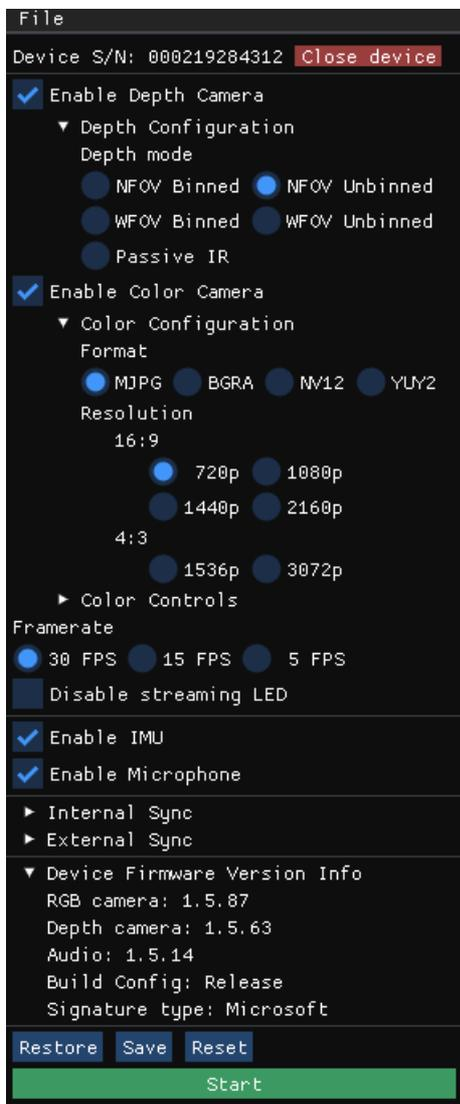
For example, in this case, the depth camera ISP is running FW 1.5.63.
