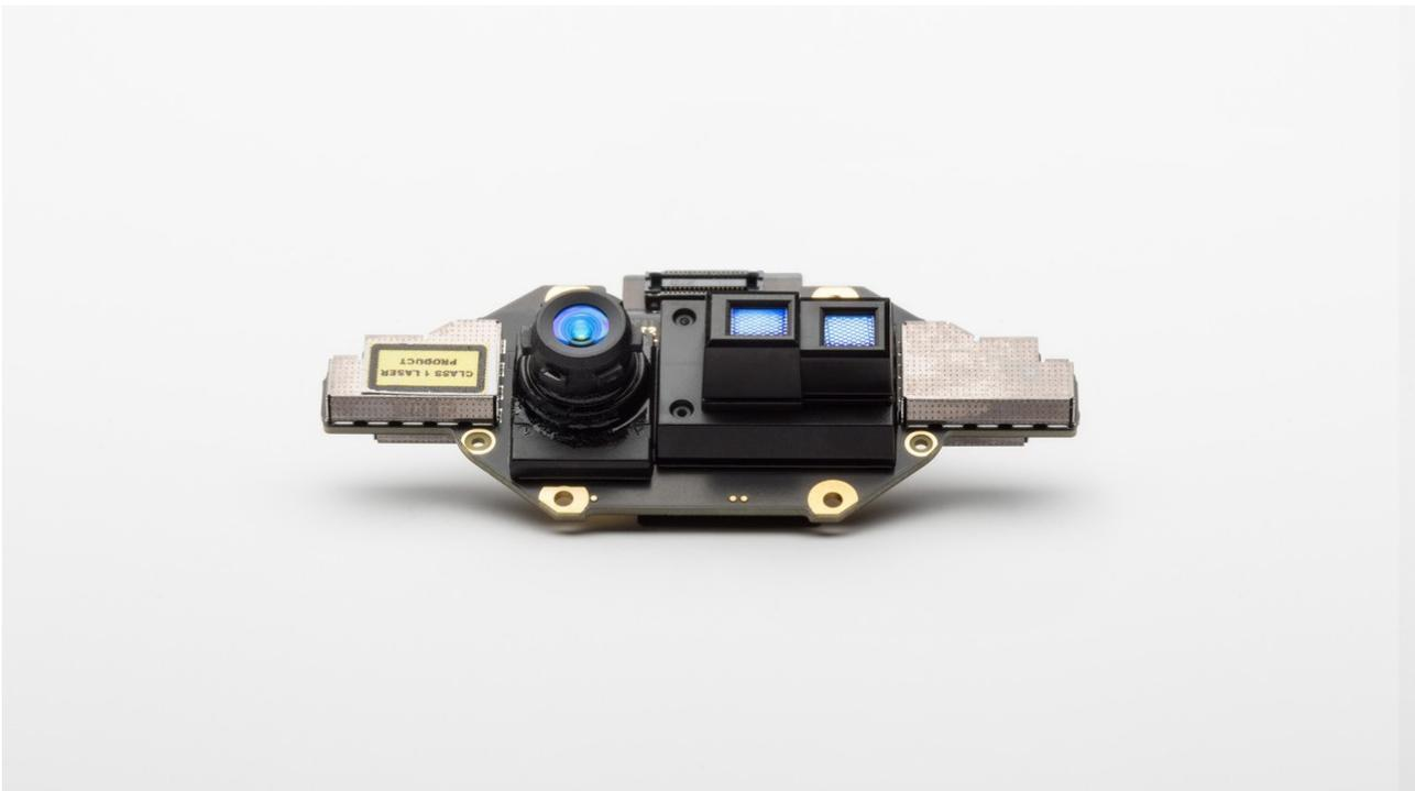
The depth camera transmits raw modulated IR images to the host PC. On the PC, the GPU accelerated depth engine software converts the raw signal into depth maps. The depth camera supports several modes. The **narrow field of view (FoV)** modes are ideal for scenes with smaller extents in X- and Y-dimensions, but larger extents in the Z-dimension. If the scene has large X- and Y-extents, but smaller Z-ranges, the **wide FoV modes** are better suited.
