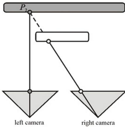
Using additional Azure Kinect DK devices will solve this issue and fill out an occlusion problem.
