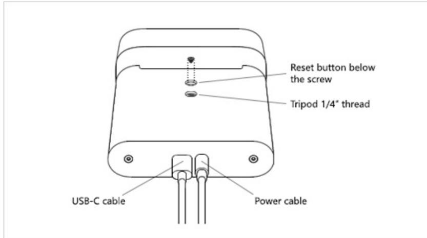
2. To find the reset button, remove the screw that's located in the tripod mount lock.
