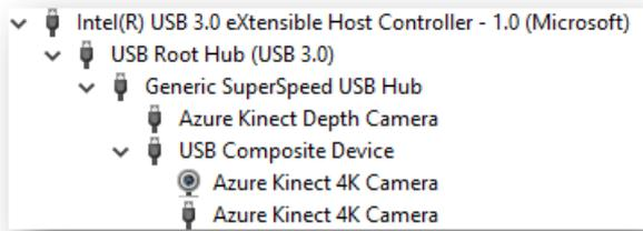
To better understand which USB port is connected on your PC, repeat these steps for each USB port as you connect Azure Kinect DK to different USB ports on the PC.
