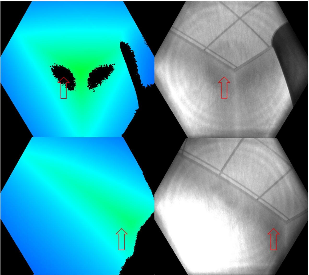
Another common case of multipath is pixels that contain the mixed signal from foreground and background (such as around object edges). During fast motion, you may see more invalidated pixels around the edges. The additional invalidated pixels are because of the exposure interval of the raw depth capture,
