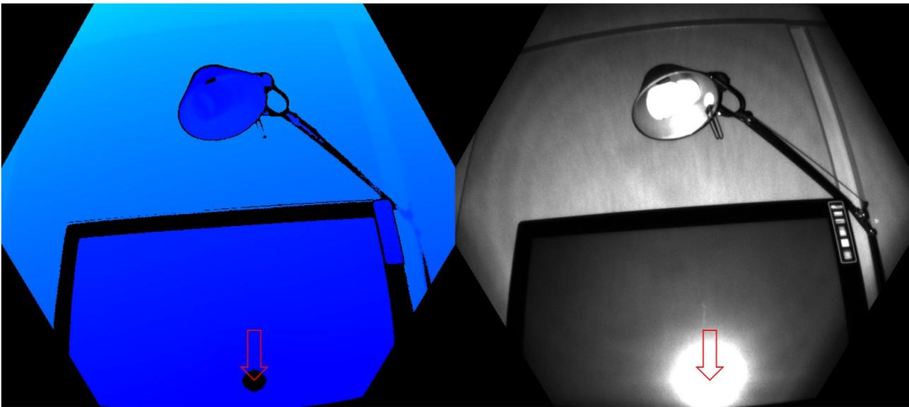
Invalidation can also occur when the IR signal isn't strong enough to generate depth. The below figure, shows the example of invalidation by a low IR signal. See the arrows pointed to example pixels in both the depth and IR images.
