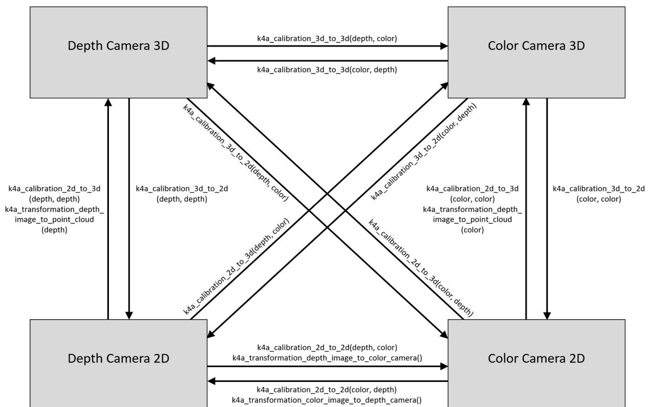
Remark on lens distortion: 2D coordinates always refer to the distorted image in the SDK. The [undistortion example](#) of the SDK demonstrates image undistortion. In general, 3D points will never be affected by lens distortion.
