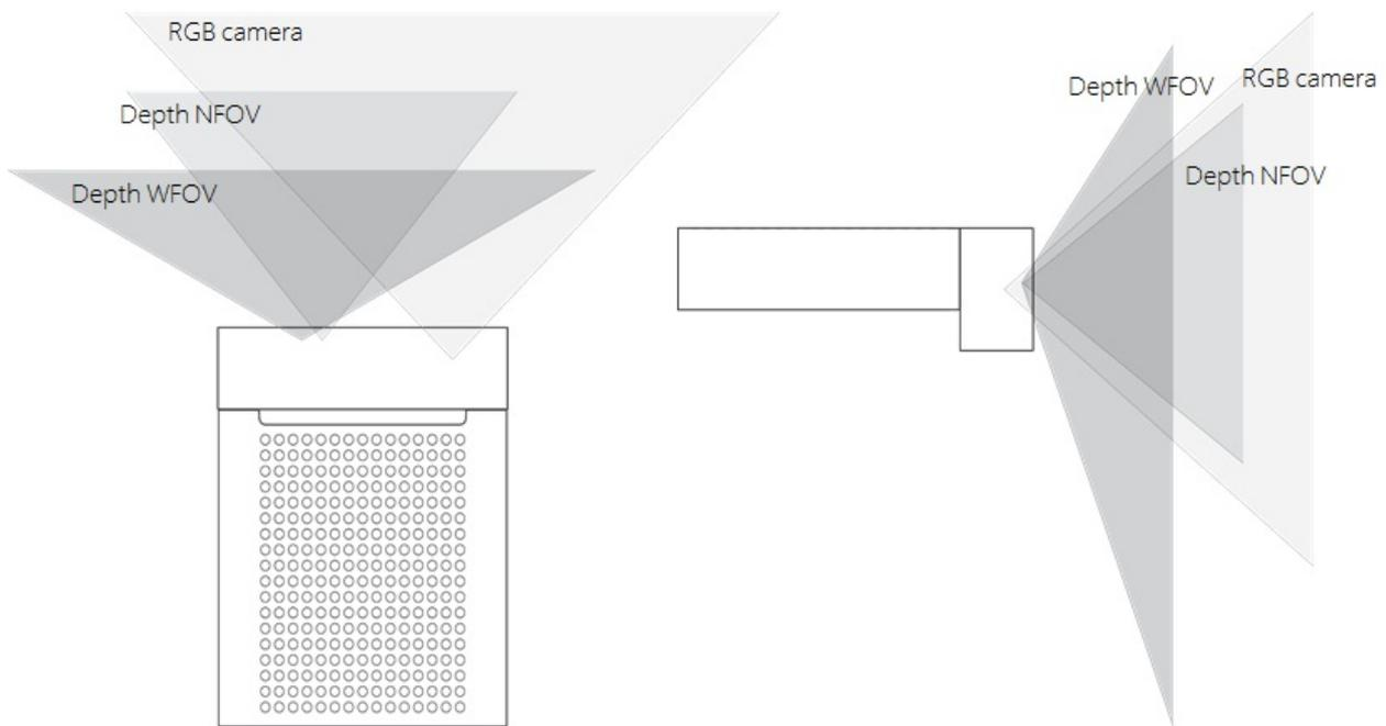
This image demonstrates the camera's field-of-view as seen from the front at a distance of 2000 mm.
